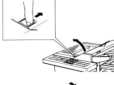
**5** Gently close the printer cover, pressing firmly on both sides of the printer cover until you hear it click.
